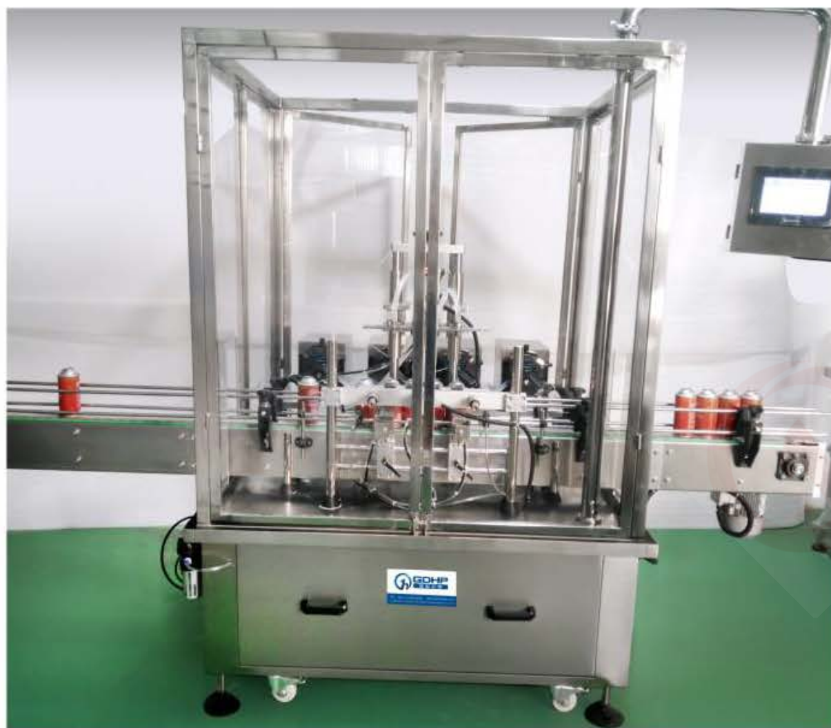
4头蠕动泵灌装机(用于各类精油, 烟油, 药液等) Auto 4-nozzle peristaltic-pump filling machine (for various oil & pharma liquids)
