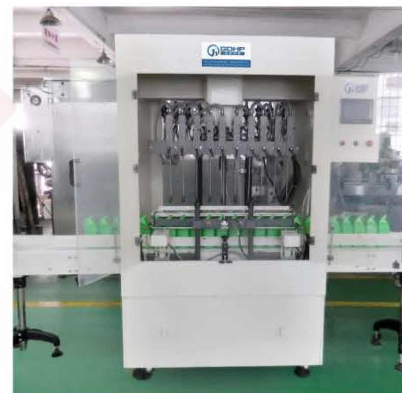
GHAGF-A10 自流式耐腐液体灌装机(用于漂白水等) Auto gravity-type anti-corrosive filling machine (for bleach etc)
