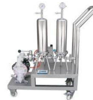
可移动式二级过滤装置 Movable secondary filtering devices
